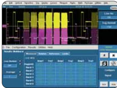
► Multiburst Measurement Results Display (Option SD and HD).
