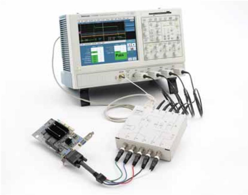
The VM5000 automates video testing of consumer HDTV and PC graphics devices such as digital set-top boxes, multi-media PCs, graphics cards and video semiconductors. It addresses the needs of engineers developing and deploying the next generation of video devices for the digitally connected home. Unrivalled performance in terms of speed, accuracy and reliability has made the VM5000 the choice of industry leaders for design validation, quality control and ATE applications.
