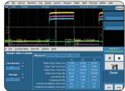
▶ RGB Transient Response Measurement Results (Option VGA).
