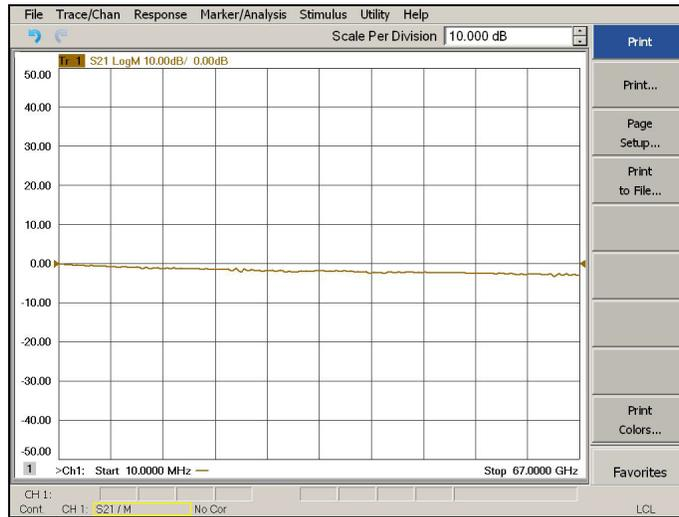
Connect the RF Flex cables to the Source IN and CPLR ARM port indicated in [Table 22](#), the expected results should be similar to [Figure 60 on page 84](#).
