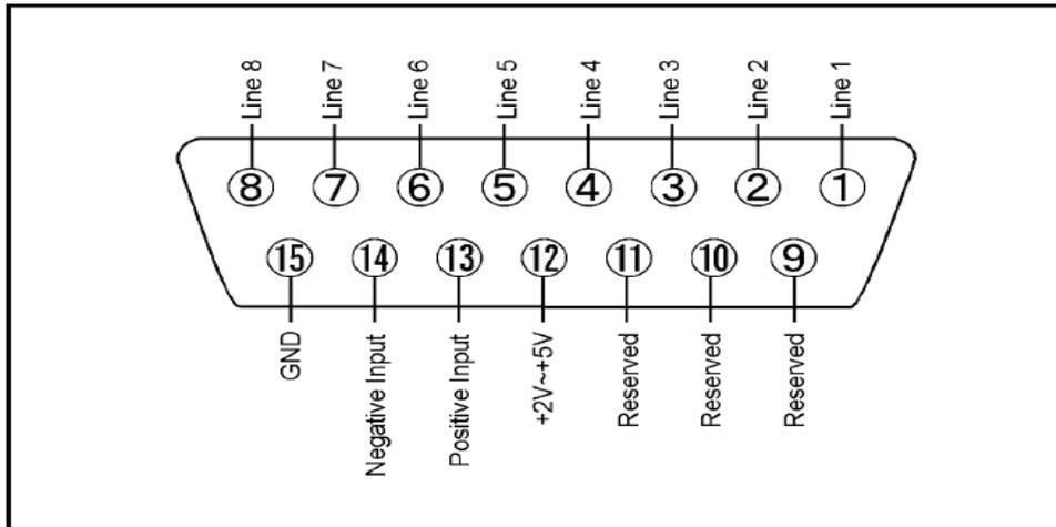
Table 12 DUT Control Line Interface Connector Pin Assignment
