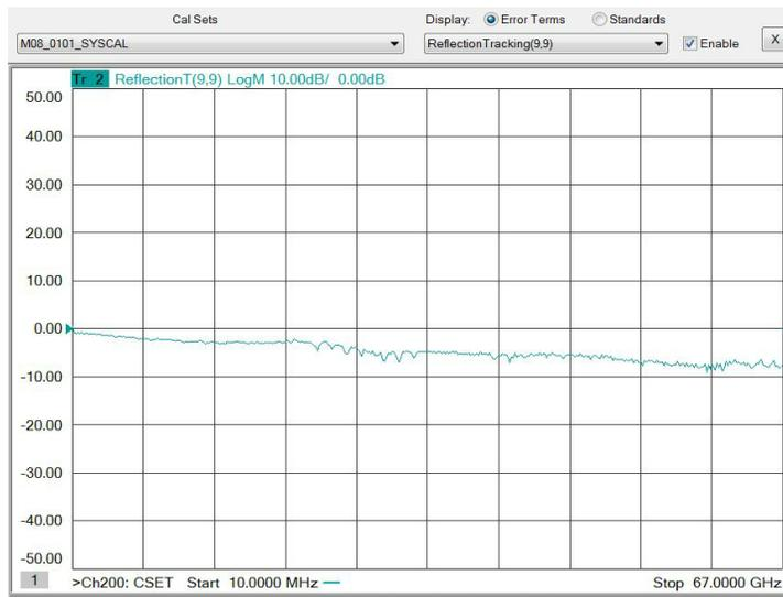
Figure 48 Typical Reflection Tracking (Ports 13 to 16)
