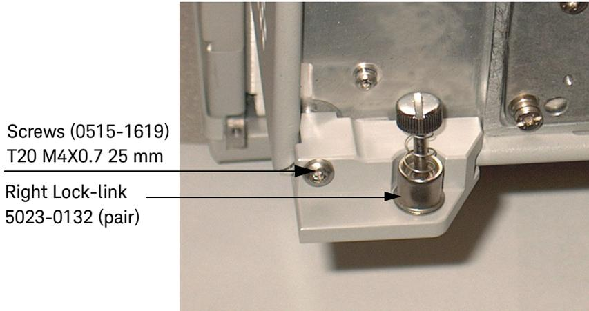
5. Remove the two upper standoffs from the rear panel of the test set using a T20 Torx driver.
