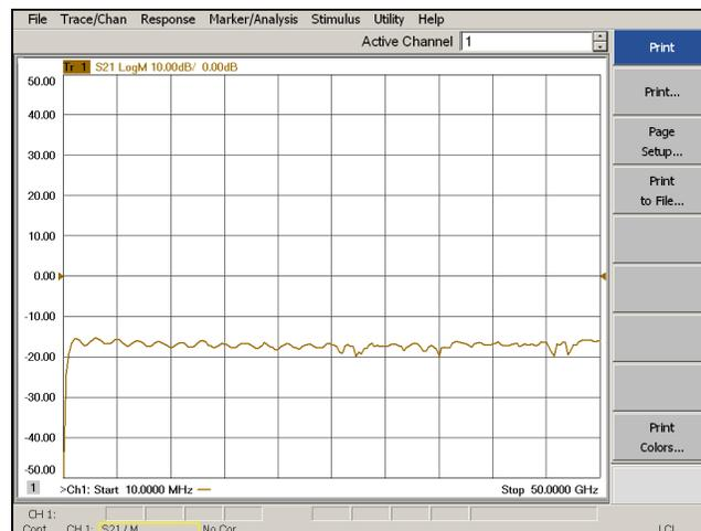
Connect the RF Flex cables to the Source IN and CPLR THRU port indicated in [Table 21](#), the expected results should be similar to [Figure 60](#).
