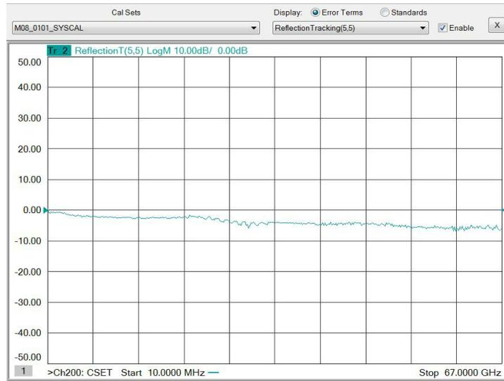
Figure 47 Typical Reflection Tracking (Ports 9 to 12)
