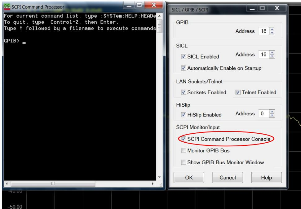
Figure 35 Command Console for 'B' Model Analyzers
