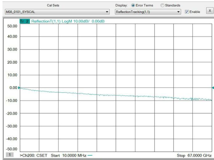
Figure 46 Typical Reflection Tracking (Ports 5 to 8)
