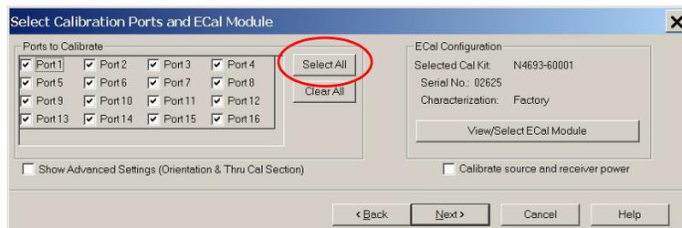
3. Connect the ECal or the mechanical cal kit to the ports you are calibrating following the Cal Wizard prompts and click **Measure** after each connection. The electrical delay value may be shown in the dialog box after the last measurement, click **OK**.
