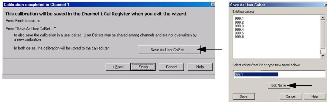
6. Repeat **step 1** thru **step 5** for Ports 2 thru 16. When finished, there should be 16 Cal Sets saved with the titles “999.1” thru “999.16” (16-Port).
