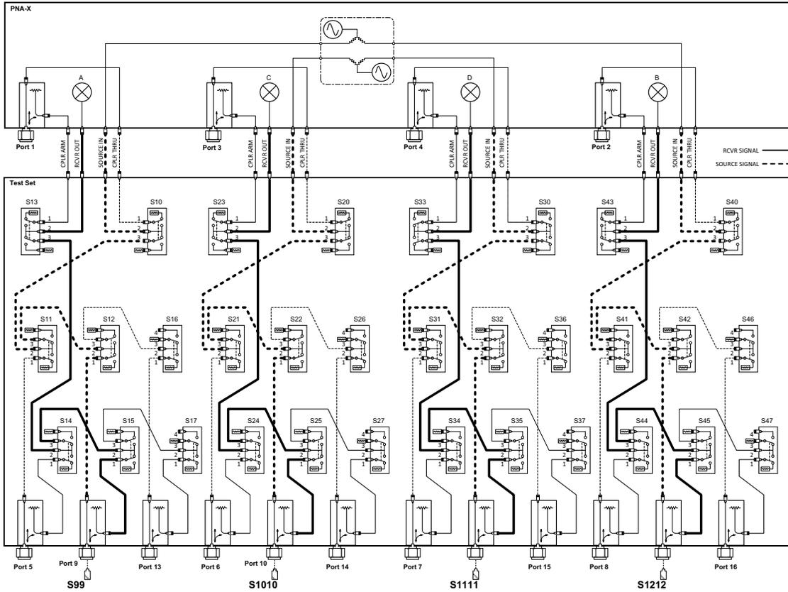
Figure 18 Typical Reflection Response Ports 13 to 16
