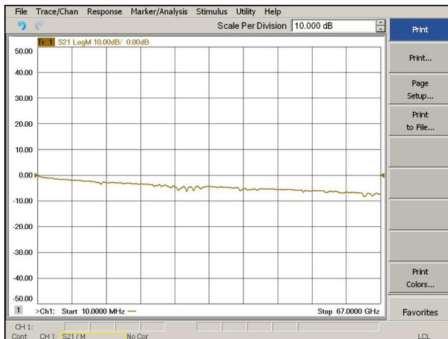
Connect the RF Flex cables to the Test Port and RCVR OUT port indicated in [Table 20](#), the expected results should be similar to [Figure 53 on page 77](#) through [Figure 55 on page 77](#).
