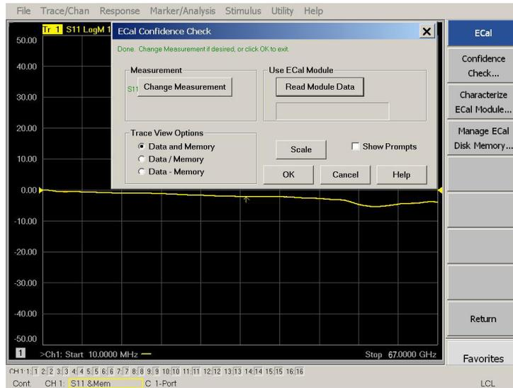
5. ECal Confidence Check dialog box: Click **Change Measurement** and select the test port **S-parameter** > **Apply** > **OK**. Click **Read Module Data**.
