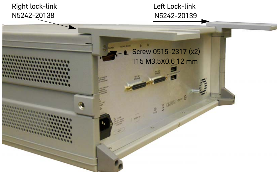
Figure 7 Install Lock-links to the Test Set
