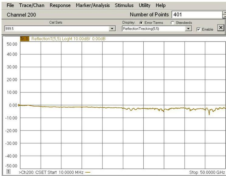
Figure 49 Typical Reflection Tracking Trace (Ports 9 to 12)
