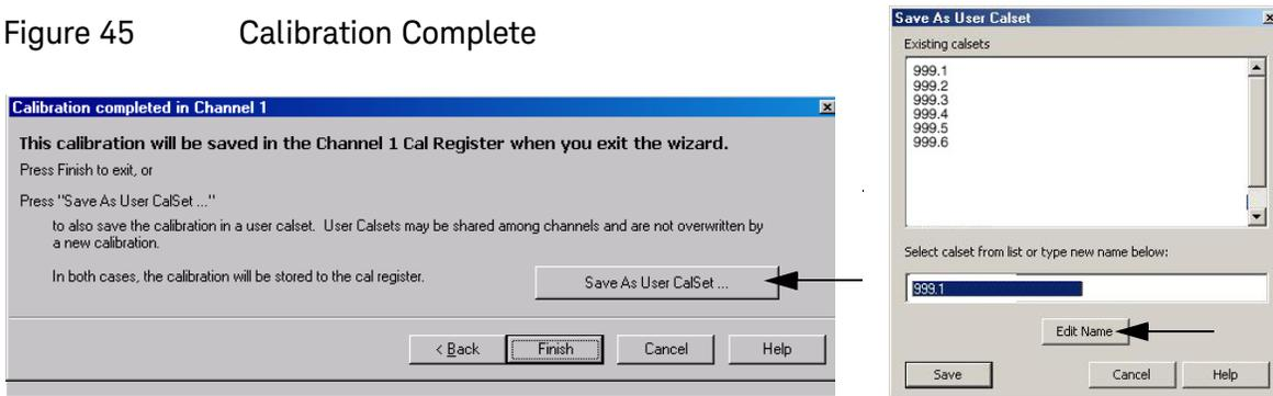
6. Repeat steps 1 thru 5 for Ports 2 thru 16. When finished, there should be 16 Cal Sets saved with the titles “999.1” thru “999.12” (12-Port).
