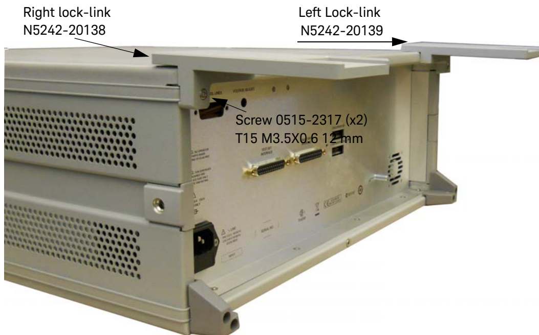
Figure 7 Install Lock-links to the Test Set
