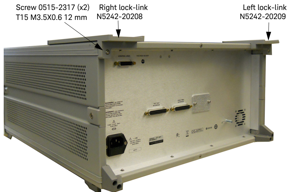
Figure 9 Install Lock-links to the Test Set
