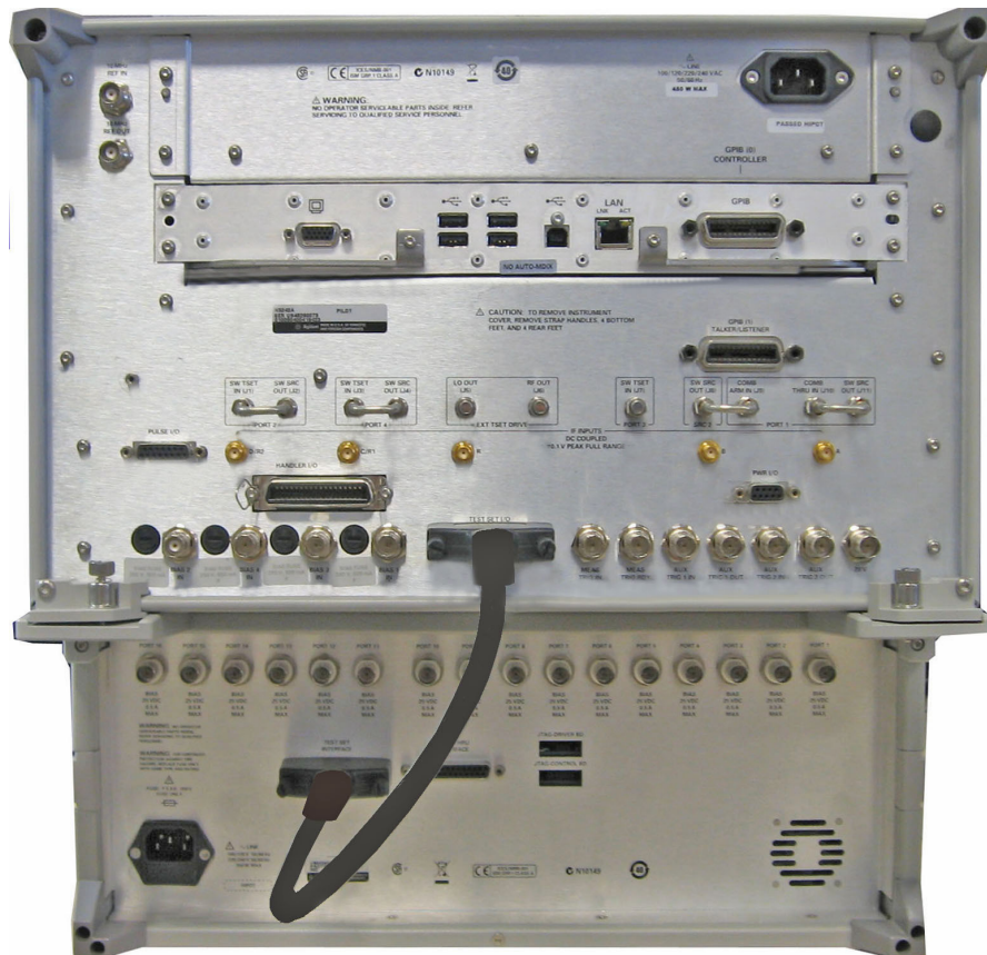
Figure 18 Test Set I/O Cable Connection
