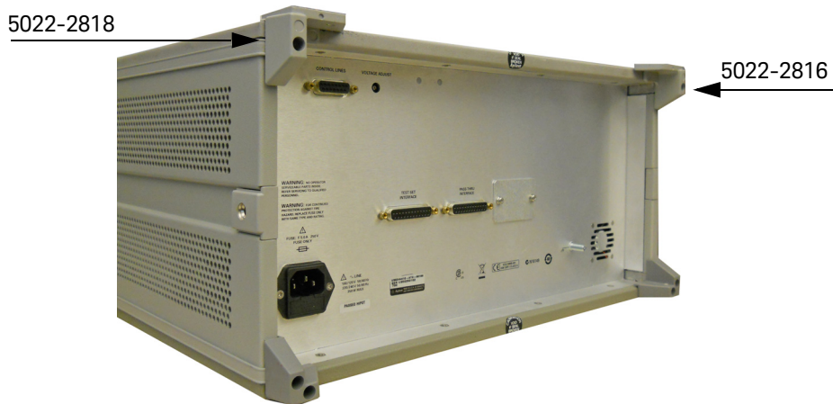
Figure 13 Installing Lock Feet on the Bottom Test Set
