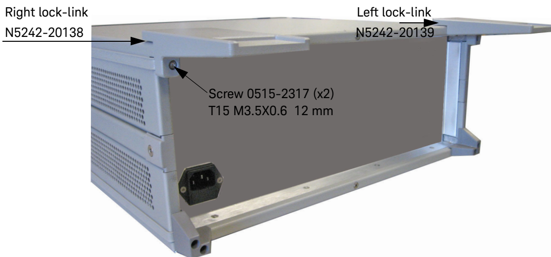
Figure 16 Install Lock-link on Test Set
