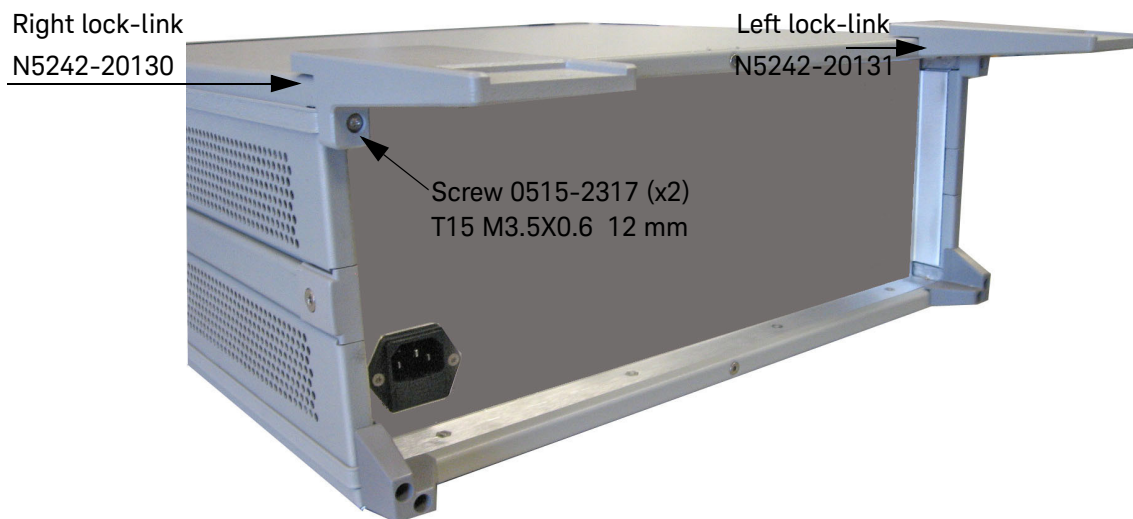
Figure 21 Install Lock-link on Test Set
