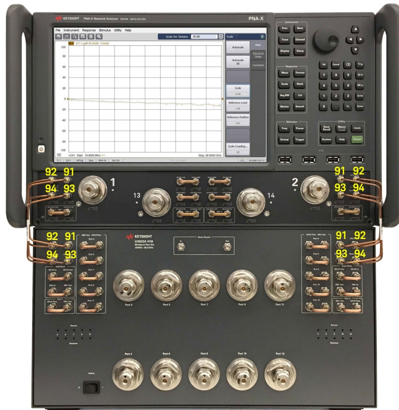
Figure 13 Rear Panel I/O Cable Configuration (Option 129)
