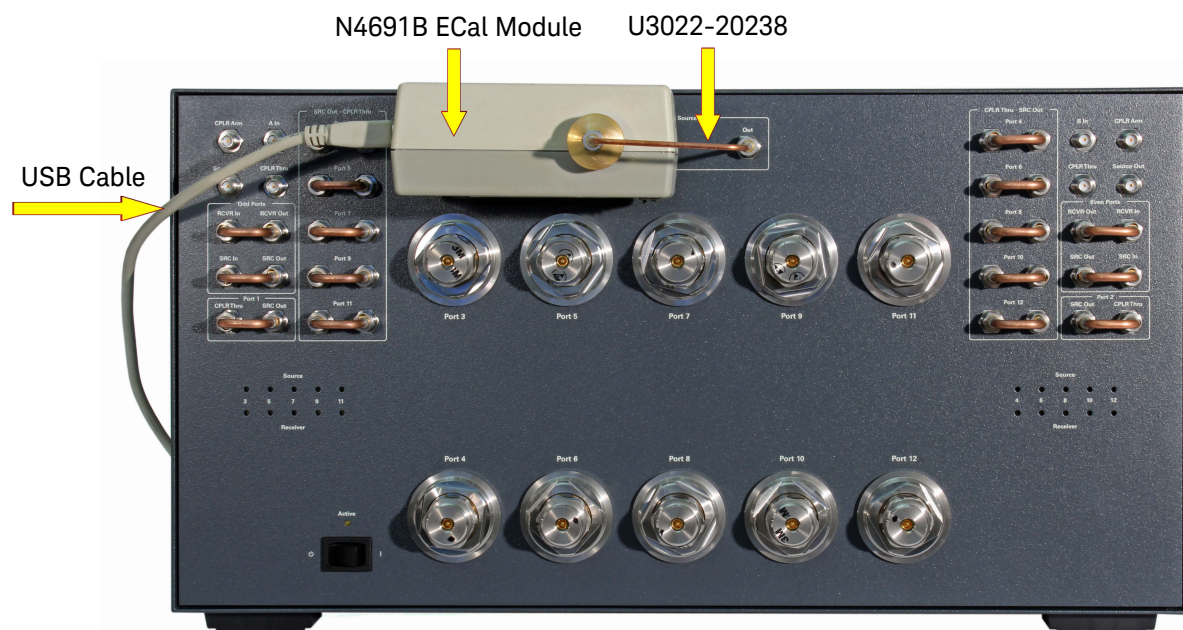
Figure 40 U3022AH10 Option 129 with ECal Module
