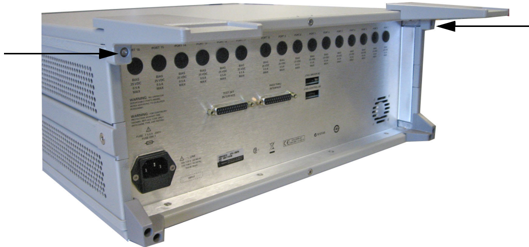
Figure 9 Install Locking Feet on U3022AH10 (STD shown)
