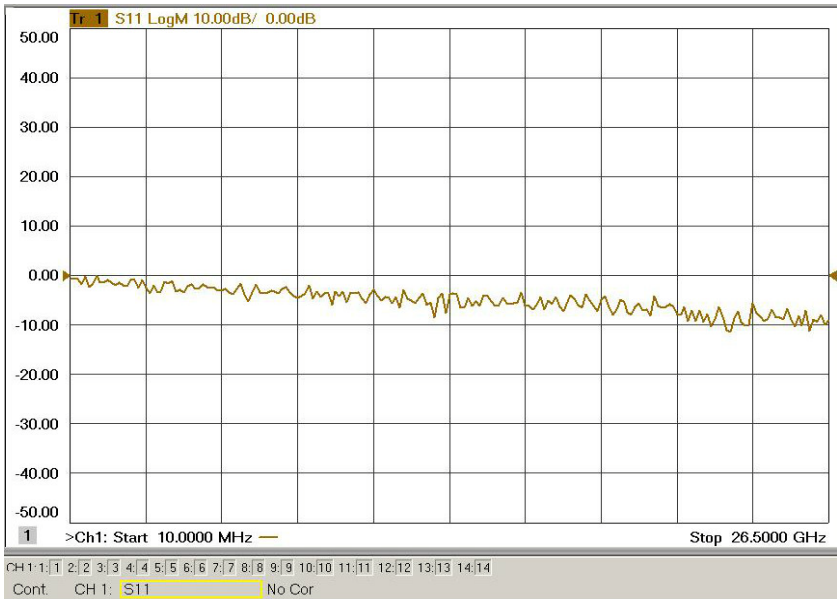
Figure 21 Typical Reflection Response Ports 1-2 (Standard)
