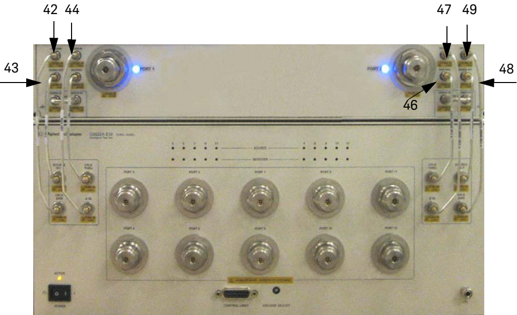
Figure 18 12-Port RF Interface Cable Connections
