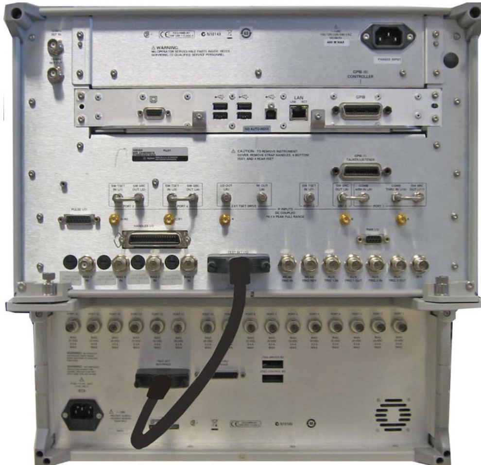
Figure 20 Test Set I/O Cable Connection
