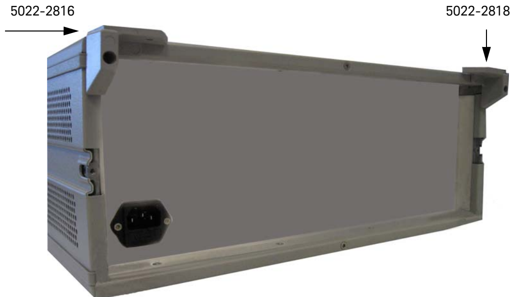
Figure 9 Install Rear Lock-links to the Test Set
