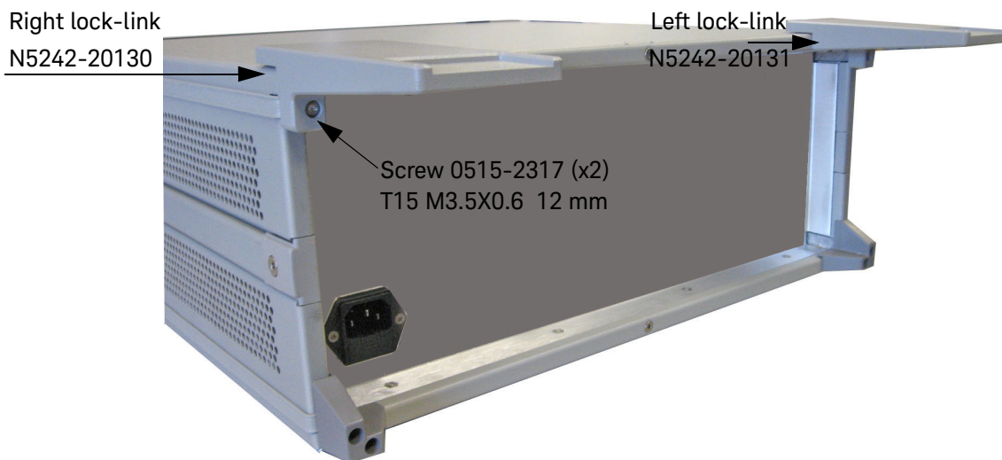
Figure 20 Install Lock-link on Test Set
