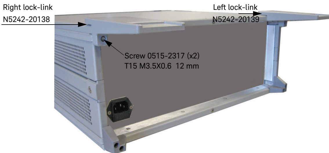
Figure 15 Install Lock-link on Test Set
