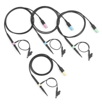
The THP0301 probes are 300 MHz, 10X passive voltage probes with 10  $\mbox{M}\Omega$  input resistance. These probes are for use with the THS3000 Series oscilloscopes and are color coded to match the oscilloscope's channel input connectors, front-panel channel selector buttons, and the displayed waveforms.
