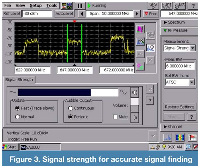
**Figure 3. Signal strength for accurate signal finding**
