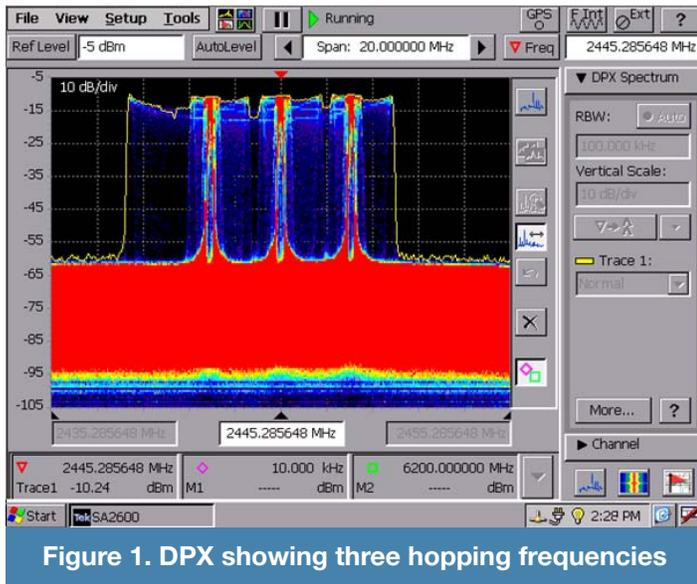
Figure 1. DPX showing three hopping frequencies
