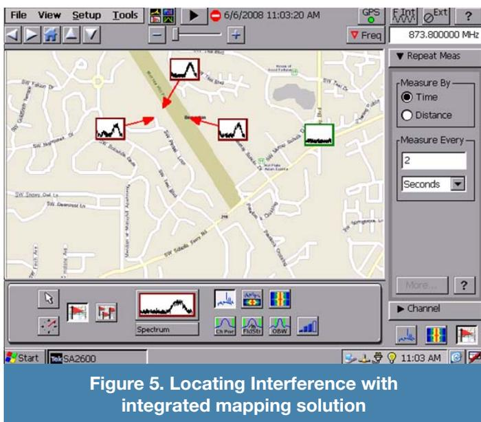
**Figure 5. Locating Interference with integrated mapping solution**
