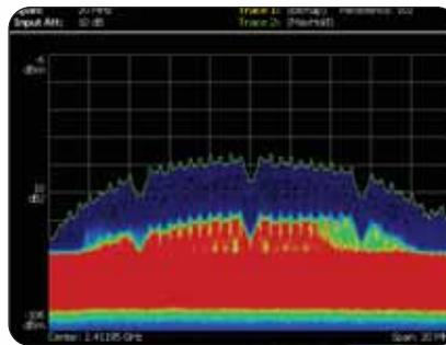
► Revolutionary DPX display discovers what other analyzers miss. Here, a WLAN Access Point and Terminal are seen transmitting at different power levels. Frequency of occurrence is color-graded, indicating that the red AP is on more often than the blue terminal.
