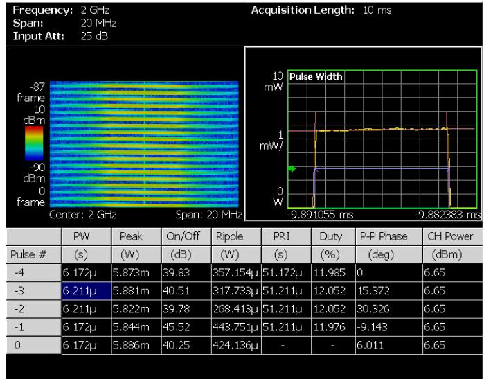
Powerful pulsed-signal analysis for characterization of Radar and other pulsed systems. Automatically measure pulse width, rep rate, pulse power, and other pulse parameters.
