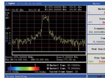
The trace display gives the view of the spectrogram for the time of the selected marker.
