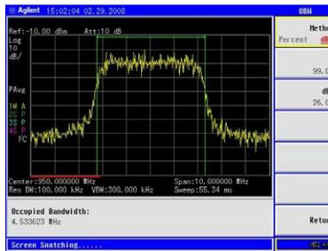
The occupied bandwidth measured in dBc.
