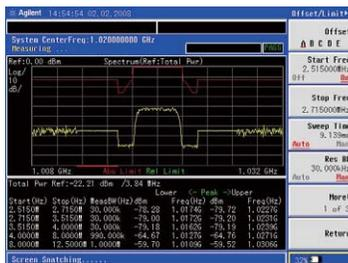
The spectrum emission mask shows the main channel power and the power level vectors relative to in-channel power for each out-of-channel frequency range.
