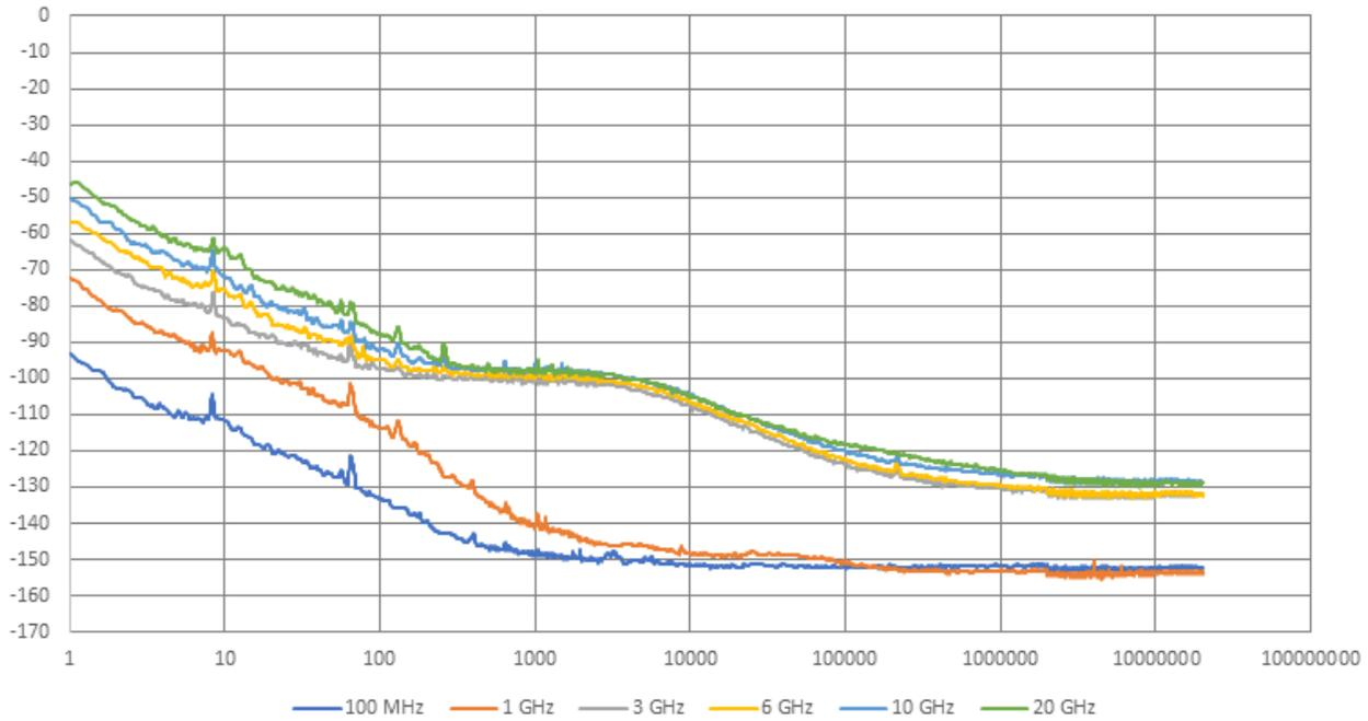
Figure 9: Measured absolute phase noise using the external LO mode for N5192A.
