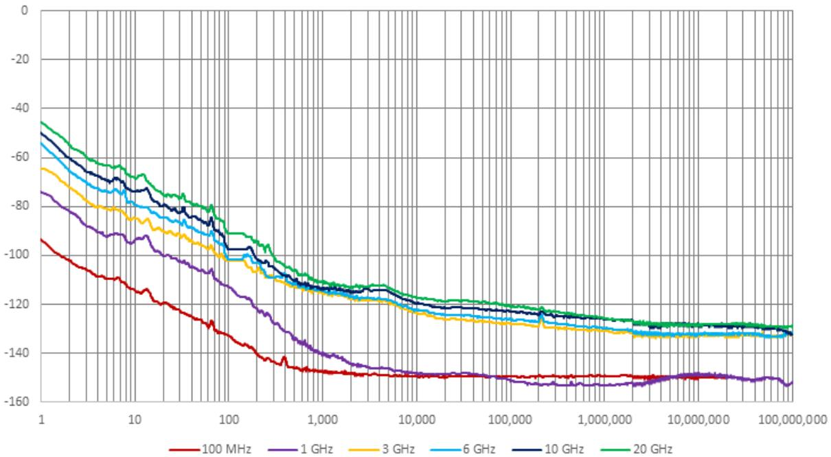
Figure 4. Measured absolute phase noise using the external LO mode for the N5194A.
