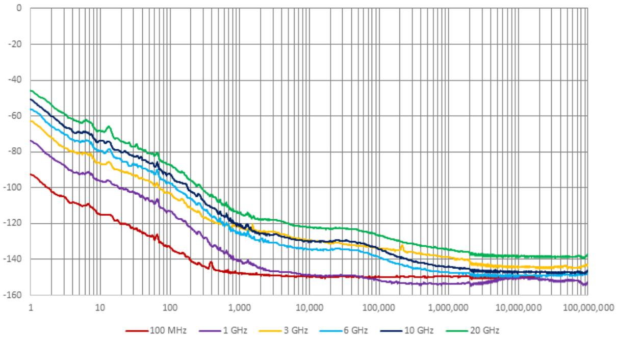
Figure 3. Measured absolute phase noise using the internal LO mode for the N5194A.
