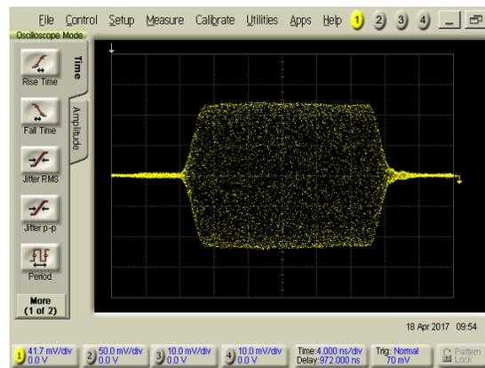
Figure 12. 20 ns pulse with 2 ns rise/fall times
