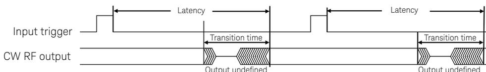
Figure 1. Switching speed definitions with input trigger
