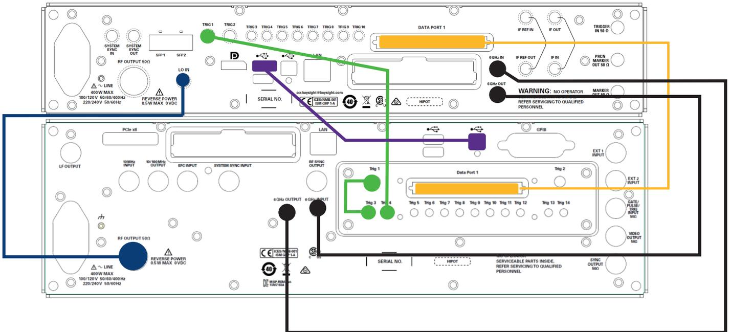
Figure 14. Connections between the UYG agile vector adapter and the UYG agile signal generator.
