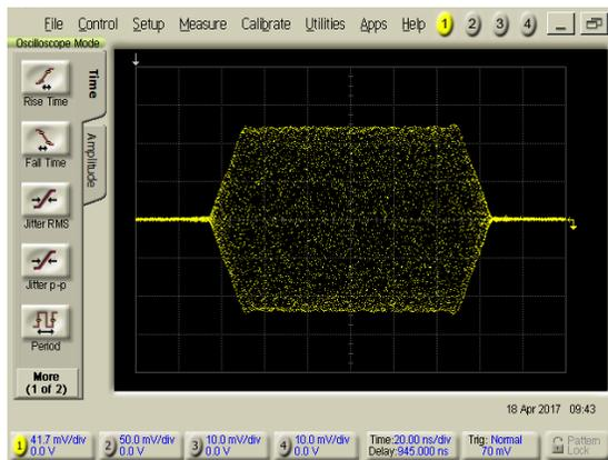
Figure 11. 100 ns pulse with 16 ns rise/fall times
