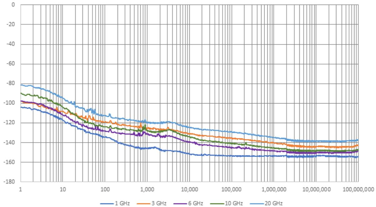
Figure 5: Measured residual phase noise using the internal LO mode for the N5194A.
