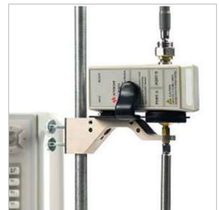
Figure 2. Ecal module connected in line for electronic calibration refresh.
