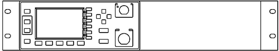
To rack mount two instruments side by side, order option 909, or lock-link kit 5061-9694 and flange kit 5063-9212.
