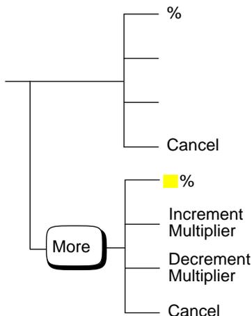
Pressing **Increment Multiplier** or **Decrement Multiplier** increases or decreases the multiplier shown in front of **%**. Pressing **%** after the correct multiplier has been selected confirms the entry.
