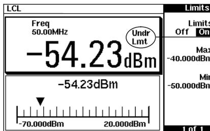
This measurement has failed as the result is less than the minimum limit level set of -50 dBm. This is indicated with the text "Undr Lmt".
