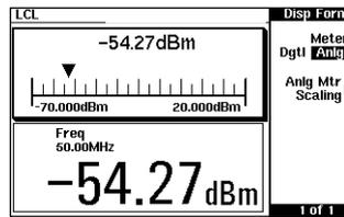
7. Press **Meter Dgtl Anlg** (Anlg should be highlighted). The upper window now displays an analog meter.
