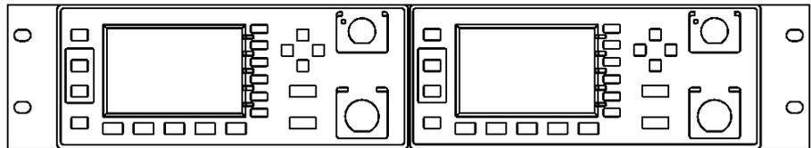
To install one or two instruments in a sliding support shelf, order shelf 5063-9255, and slide kit 1494-0015 (for a single instrument, also order filler panel 5002-3999).
