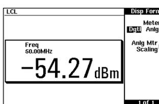
4. Press **Meas Setup**, **Display Format**, **Meter Dgtl Anlg** (Dgtl should be highlighted). The display shows a digital window.
