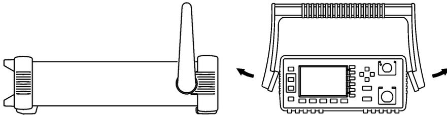
2. Remove the rubber bumper by stretching a corner and sliding it off.
