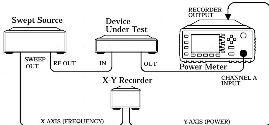
To access the “Recorder” menu press **System Inputs**, **More**, **Recorder Output**. This menu allows you to switch the Recorder Output signal either on or off. The **Max Power** and **Min Power** softkeys allow you to enter the input power level that you want to represent the 1 V<sub>dc</sub> maximum and 0 V<sub>dc</sub> minimum output voltage of the Recorder Output.
