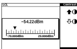
3. Press **Left/Right**. The display now only shows the one window. This is the analog window which, in the previous step was selected with the **Up/Down** key.
