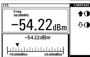
2. Press **Up/Down**. The display remains the same apart from the fact that it is now the lower window (which is an analog display) that is highlighted by the dark box.
