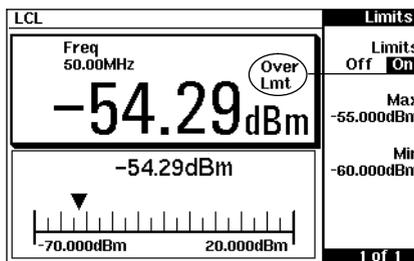
This measurement has failed as the result is more than the maximum limit level set of -55 dBm. This is indicated with the text "Over Lmt".
