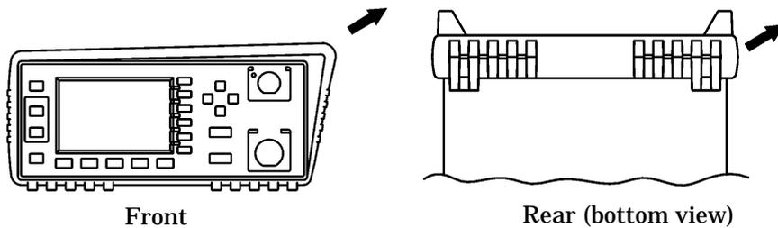
To rack mount a single instrument, order option 908, or adapter kit 5063-9239.
