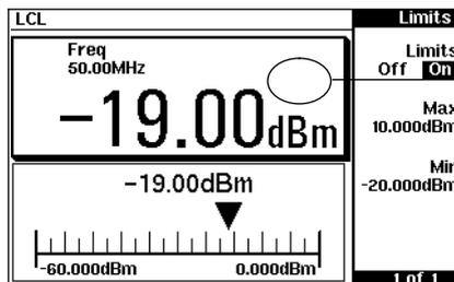
This measurement has passed. This is indicated by the limit field being empty.
