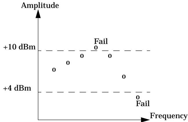
In this application a swept frequency signal is applied to the input of the Device Under Test. The power meter measures the output power. The limits have been set at +4 dBm and +10 dBm. A fail occurs each time the output power is outside these limits as shown in Figure 2-7.
