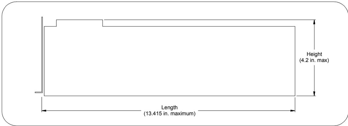
**Figure 6-4. I/O Board Dimensions for E985xA Expansion Slot**
