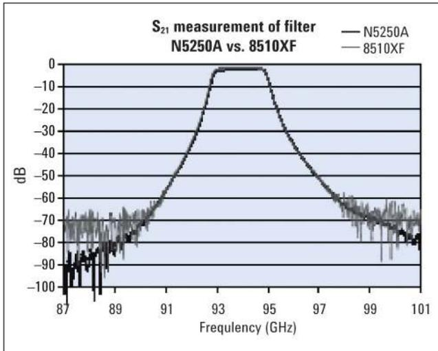
The N5250A PNA-based mmwave system has superb dynamic range. Shown here is the S<sub>21</sub> of a filter at 94 GHz, compared to the 8510XF.
