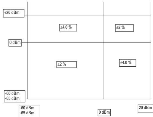
Figure 5 shows the typical uncertainty in making a relative power measurement, using the same power meter channel and the same power sensor to obtain the reference and the measured values. It also assumes that negligible change in frequency and mismatch error occurs when transitioning from the power level used as the reference to the power level measured.
