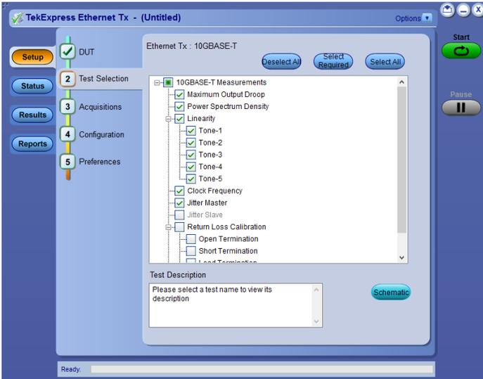
**TekExpress Ethernet Tx (Option XGBT2)** – Quickly perform 10GBASE-T measurements per the IEEE 802.3an-2006 standard including Power Spectral Density (PSD), Power Level, and Linearity, with a simplified instrument configuration. XGBT2 provides flexible control over test configurations and analysis parameters, enabling more in-depth device characterization.
