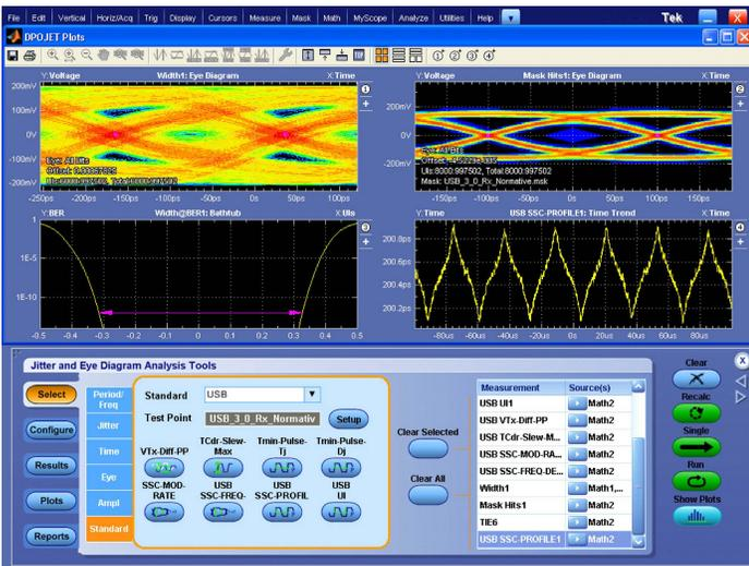
**USB 3.0 Transmitter Test Solution (Option USB3)** – Perform verification, characterization, and debug of USB 3.0 devices. Measurements are implemented in DPOJET and are compliant to the USB 3.0 specification. For compliance and automation, USB-TX is available.
