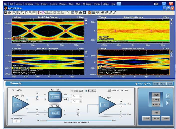
**SDLA - Serial Data Link Analysis Visualizer (Option SDLA64)** – Offers the capability to emulate the serial data channel, de-embed fixtures, cables, or probes, and add or remove equalization. Option SDLA64 also provides processing of waveforms with IBIS-AMI Receiver Equalization, or CTLE, FFE and/or DFE equalization. DPOJET provides advanced measurement and jitter analysis of the resulting waveforms.
