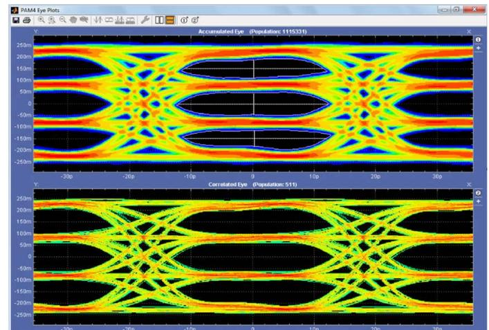
**NRZ and PAM4 measurements**–The throughput of Datacom networks continues to increase. Tek's DPO73304DX supports up to 10GBASE-KRn data rates. The powerful combination of the DPO70000, DPOJET Jitter and Noise Analysis, and the SDLA Serial Data Link Analysis tool performs accurate de-embedding and eye diagram analysis for Datacom standards.
