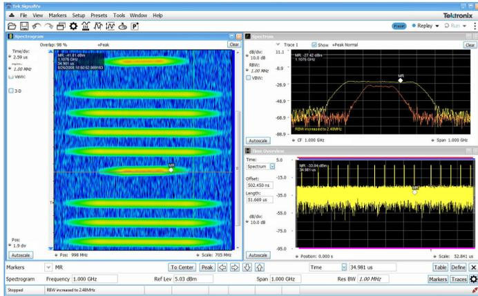
SignalVu® Vector Signal Analysis – Easily verify wide-bandwidth designs such as wideband radar, high data-rate satellite links, WLAN 802.11, or frequency-hopping radios and characterize wideband spectral events. SignalVu® combines the functionality of a vector signal analyzer, a spectrum analyzer, and the powerful triggering capabilities of the MSO/DPO70000 Series – all in a single package.
