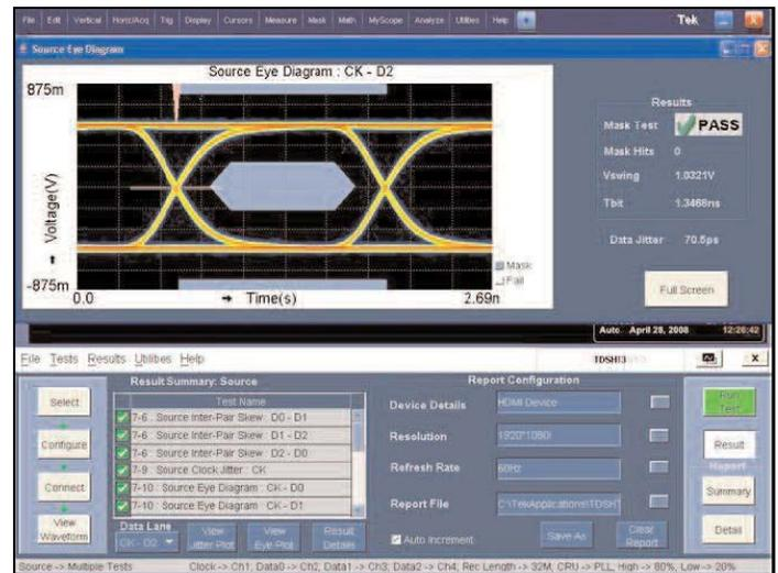
**HDMI Compliance Test Solution (Option HT3)** – A fast, efficient solution for HDMI compliance measurement challenges, no matter if you are working on a Source, Cable, or Sink solution. This application provides all the HDMI compliance test solutions you need to ensure quality and interoperability.
