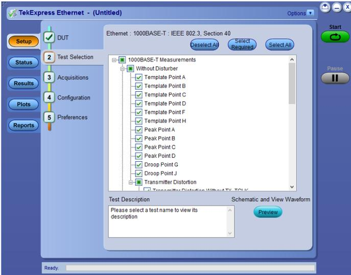
**TekExpress Ethernet (Option CMENET3)** – Receive full PHY layer support for Ethernet variants 10BASE-T, 100BASE-TX, and 1000BASE-T with the comprehensive, integrated Tektronix® TekExpress Ethernet tool set. Analog verification, automated compliance software, and device characterization solutions are all included.
