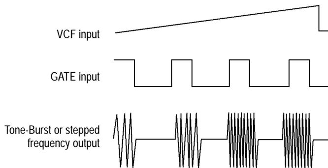
**Figure 9: Tone-Burst and Stepped Frequency Typical Waveforms**
