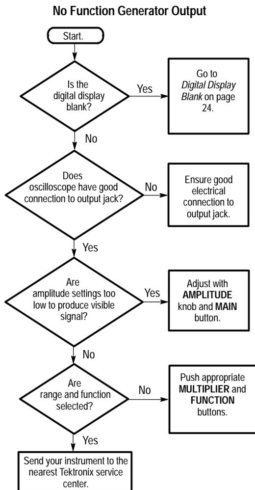
**Inappropriate Function Generator Output**
