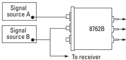
Figure 4. Multi-source switching
