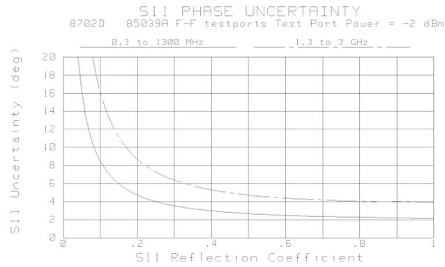
**System E/E Characteristics****Agilent 8702D (75Ω) using Agilent 85039A M-M Test Ports****MEASUREMENT PORT CHARACTERISTICS (CORRECTED)<sup>a</sup>
