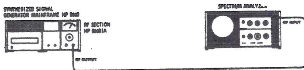
Figure 4-5. Harmonic Signal Test Setup
