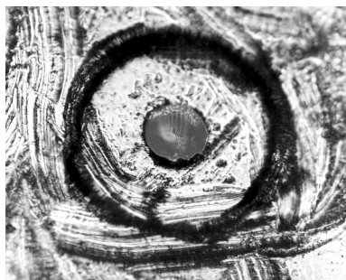
Figure 8-6. Damage from improper cleaning.
