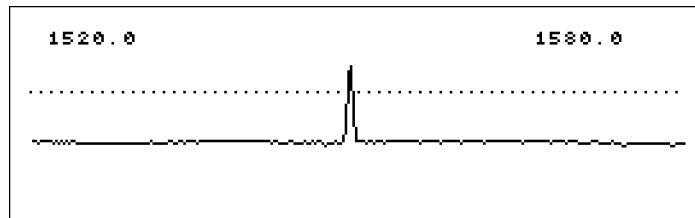
PRBS modulation graph showing raised noise floor.
