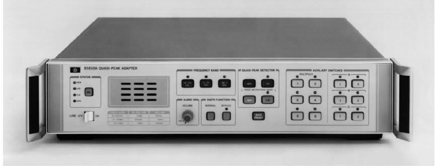
The bypass mode returns the spectrum analyzer back to standard operation unaffected by the quasi-peak adapter. In the normal mode the three CISPR bandwidths are available and the quasi-peak detector can be turned on and off.
