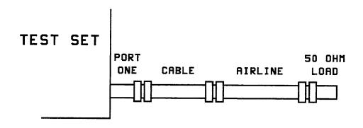
Figure 1. Return Loss Set-up
