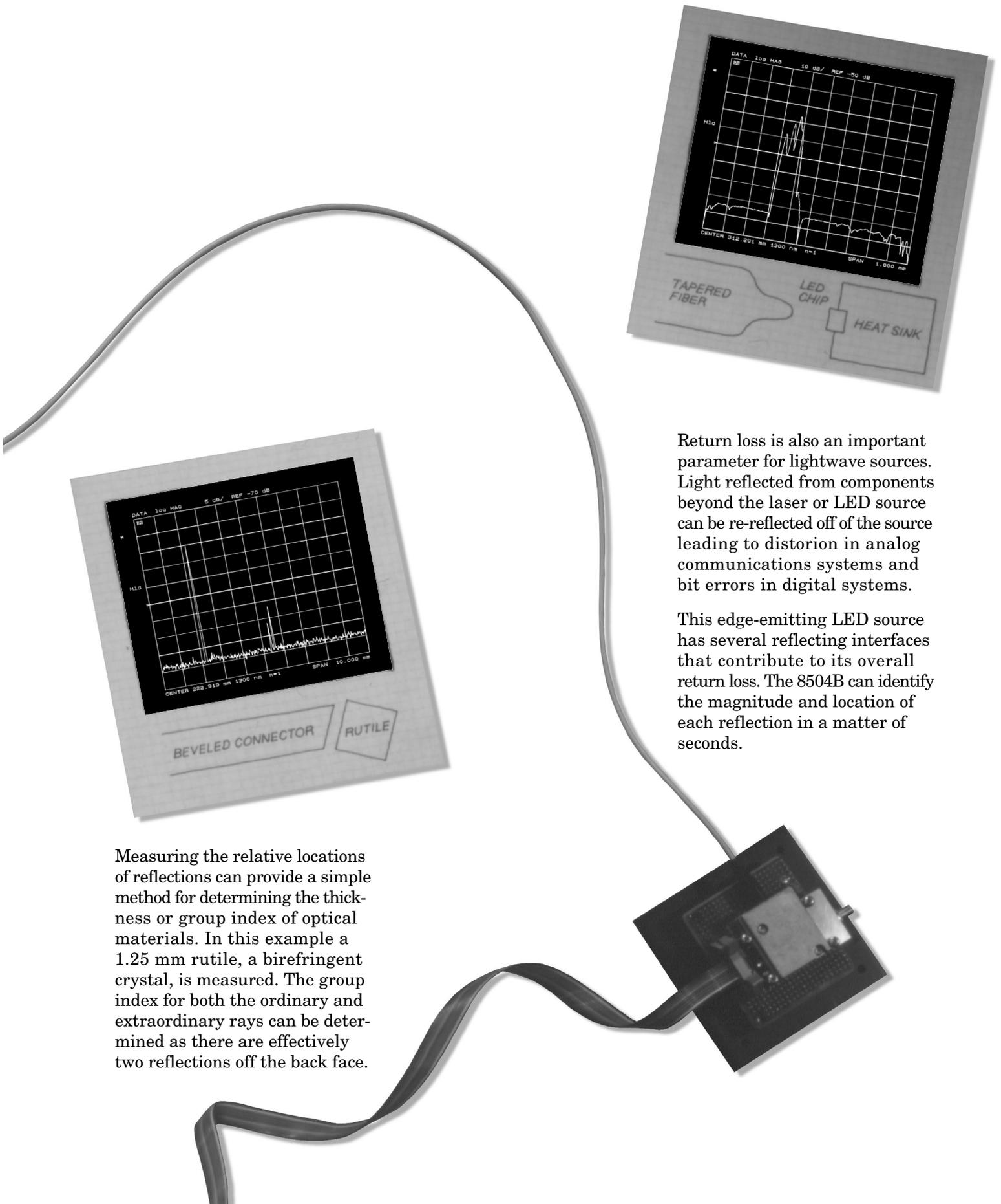
Return loss is also an important parameter for lightwave sources. Light reflected from components beyond the laser or LED source can be re-reflected off of the source leading to distortion in analog communications systems and bit errors in digital systems.
