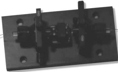
The total return loss of this photodiode assembly is due to several different interfaces. The 8504B precision reflectometer shows the return loss of each of the photodiode's elements. Designers no longer need to guess where to concentrate their efforts in improving the product.
