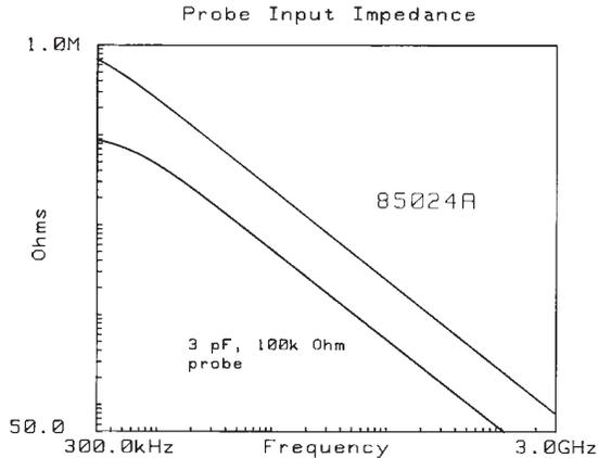
Probe with less error due to higher input impedance. For example, in a 50 ohm system at 500 MHz, the 85024A presents 455 ohms which produces a 10% signal loss from loading effects, while a 3 pF, 100 kΩ probe presents 106 ohms causing a 32% signal loss.
