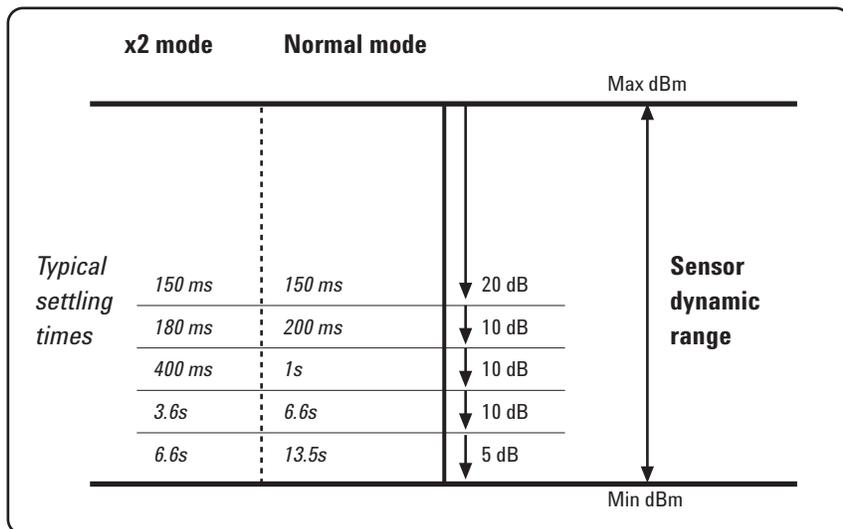
1. Settling time: 0 to 99% settled readings over the GPIB
