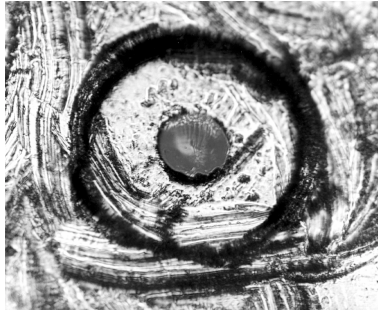
Figure 3-7. Damage from improper cleaning.
