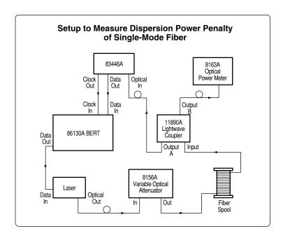
Certain industry standards such as SONET and Fibre Channel require that the eye diagram be measured through a reference receiver having a carefully-controlled frequency response. In this case, the Agilent 83446A can be used to recover the clock and a separate reference receiver used to display the eye diagram.
