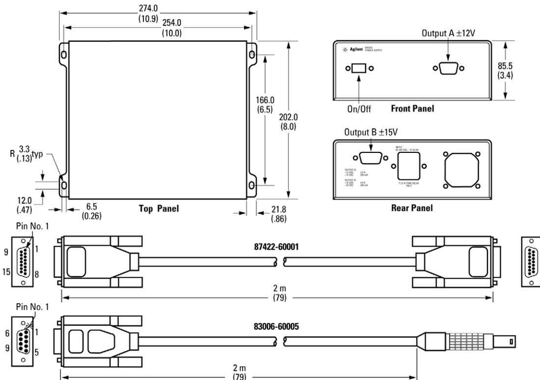
The 87422A power supply provides the dc power needed to bias the 8302A, plus an additional  $\pm 12V$  dc output.
