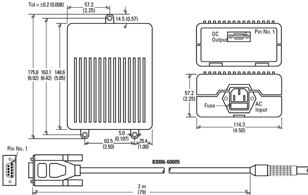
The 87421A power supply provides the dc power needed to bias the 83006A, 83017A, 83018A, 83050A, and 83051A.
