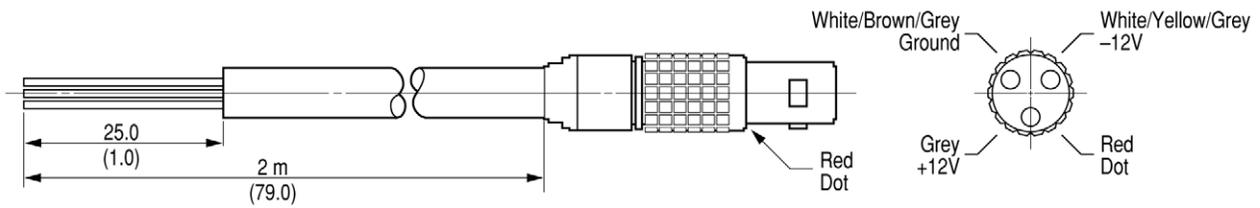
83006-60004 dc bias cable. Cable shipped with 8300A, 83017A, 83018A, 83050A, and 83051A.
