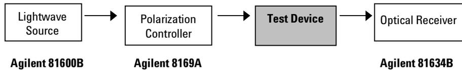
Figure 1: Conceptual block diagram of polarization measurements.
