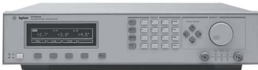
Agilent's 8169A Polarization controller enables automatic polarization state adjustments for measurements of polarization dependent loss (PDL) and polarization mode dispersion (PMD), and for polarization synthesis applications.
