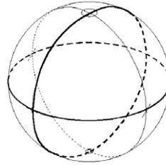
Figure 2: Orthogonal circles on the Poincare sphere<sup>1</sup> show how the Agilent 8169A synthesizes relative state-of-polarization points according to a specified path.
