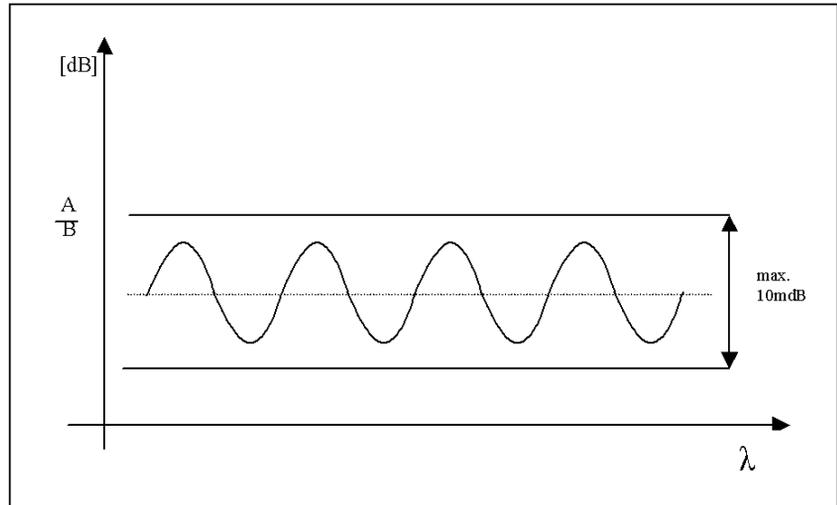
Figure 15 Interference Ripple
