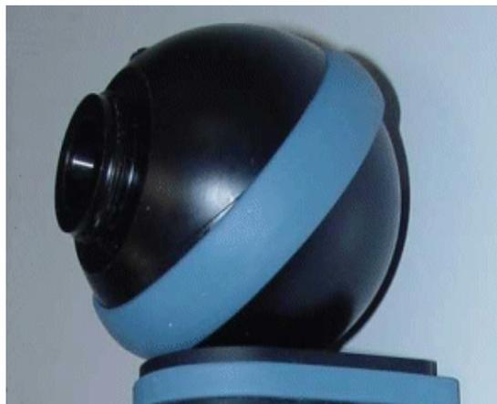
Figure 4 Attaching the Rubber Ring
