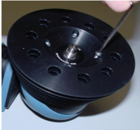
Figure 6 Attaching the Upper Part of the Heat Sink
