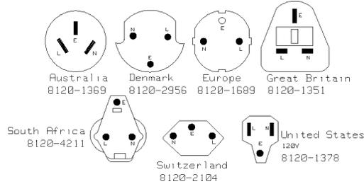
**Figure A-1. Line Power Cables - Plug Identification**
