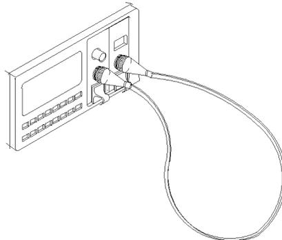
**Figure 3-1. Measuring the Reference for the Loss Application**
