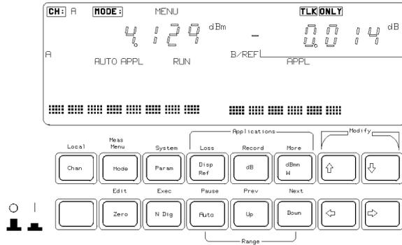
**Figure 3-11. The Display during the Alignment Application**
