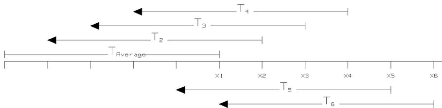
**Figure 8-2. Measurements with  $T_{Average} > 1$  second, continuous triggering.**
