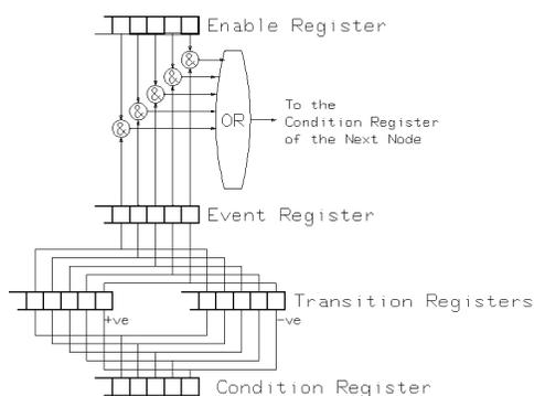
**Figure 7-1. The Registers and Filters in a Node**
