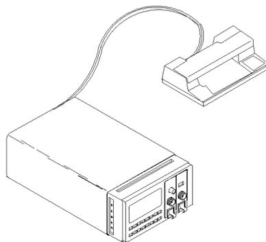
**Figure 1-9. A Plotter Connected to the HP 8153A**
