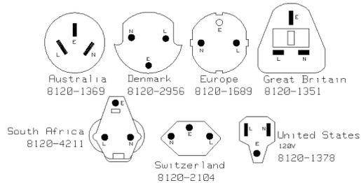
**Figure 0-1. Line Power Cables - Plug Identification**
