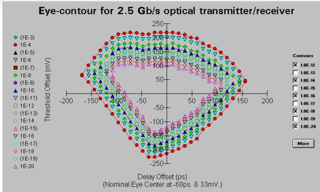
Use HP E4543A application software to derive eye contours to  $10^{-20}$  BER from Q measurement.
