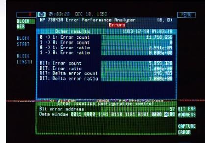
Error location analysis has identified bit 57 of a long, repetitive pattern to be in error. The preceding 28 bits and three following bits are also displayed. The separate analysis of 1→0 and 0→1 errors helps you locate sources of errors. If you need to view more of the pattern that may have caused the error, the pattern editor is on hand to let you view all of the pattern.
