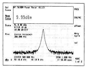
The Modular Measurement System allows you to customize your CRT to display up to 4 instruments at one time. In the picture at left, an HP 70100A Power Meter Module is displayed in the top window and a spectrum analyzer is displayed in the bottom window.
