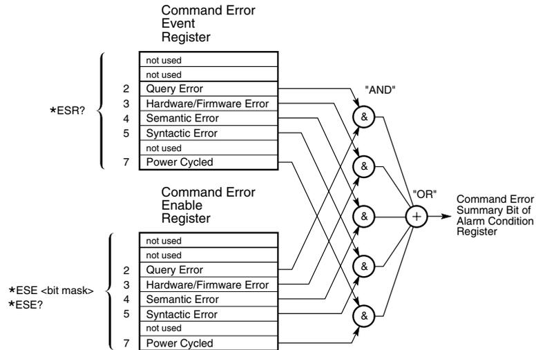
Figure 5-4. Command Error Event and Enable Registers
