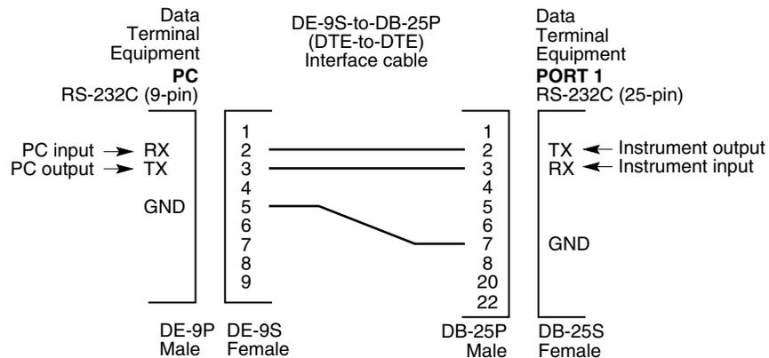
**Figure 2-4 DE-9S-to-DB-25P (DTE-to-DTE) Serial Interface Connection to PORT 1**
