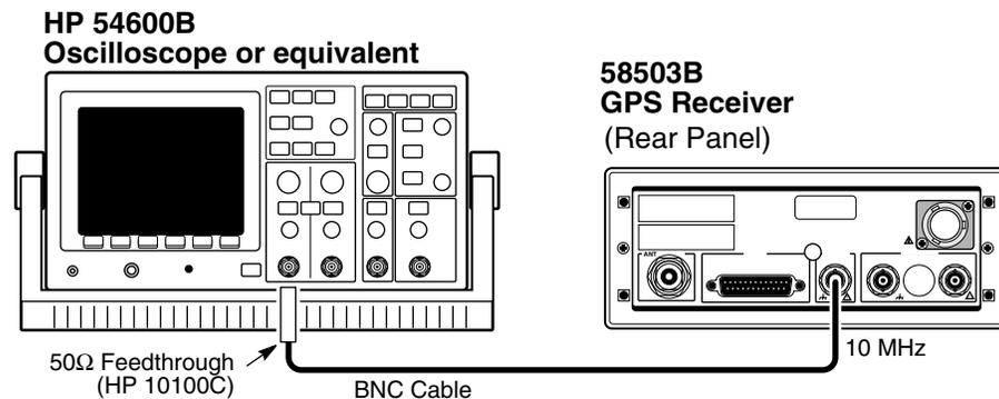
**Figure D-1. 58503B 10 MHz Operational Verification Setup**
