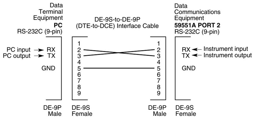
**Figure 2-3 DE-9S-to-DE-9P (DTE-to-DCE) Serial Interface Connection to PORT 2**
