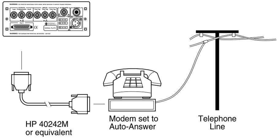
**Figure 2-2 Connecting the GPS Receiver to a Modem**
