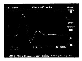
With a 1 gigasample/second digitizing rate, the HP 54111D captured this laser pulse single-shot.
