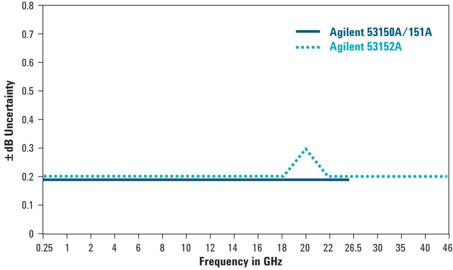
Figure 1. -10 dBm input level at 25 °C
