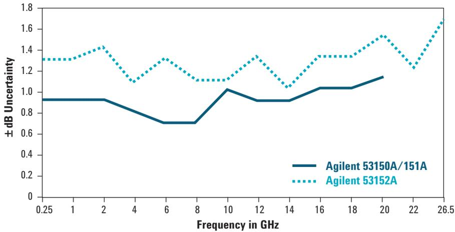
Figure 4. -25 dBm input level from 0 to 55 °C
