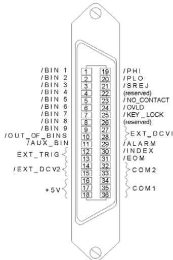
Figure 7. Pin assignment of the handler interface connector
