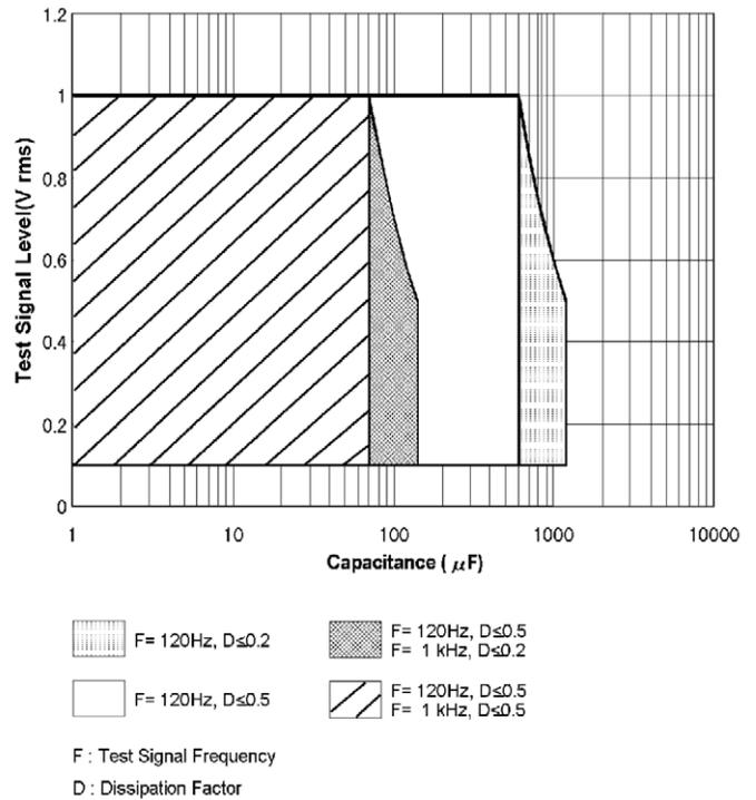
Figure 4. Operating range of the ALC function
