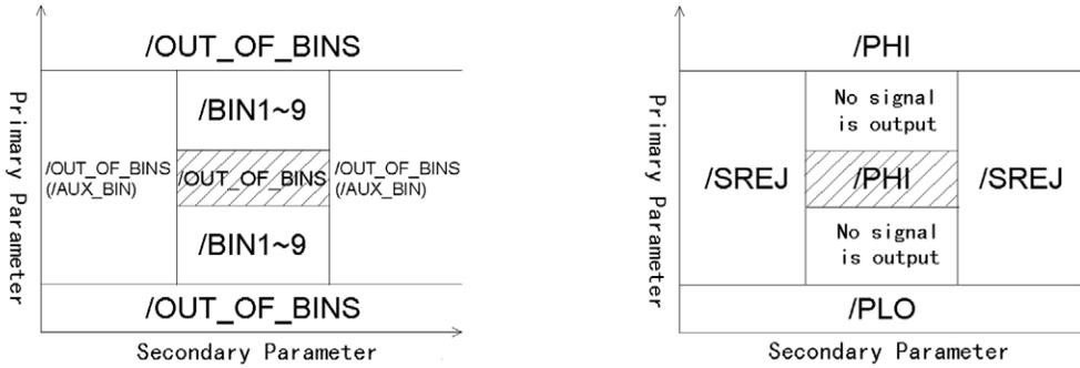
Signals encircled with ( ) are outputted when the AUX BIN function is ON.
