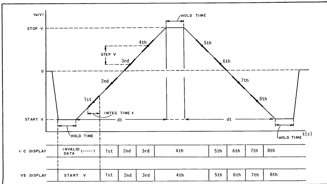
Figure 3-19. Relationship between C-V Measurement and Displays for  $\nabla$  (Double Ramp Wave).
