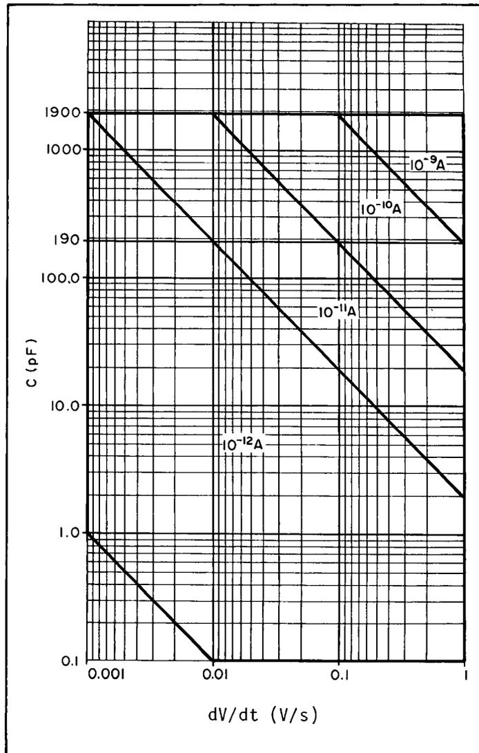
Figure 3-21. Suitable Current Ranges for C-V Measurements,
