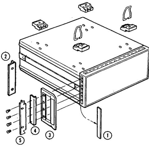
1. Remove adhesive-backed trim strips (1) from sides at right and left front of instrument.
