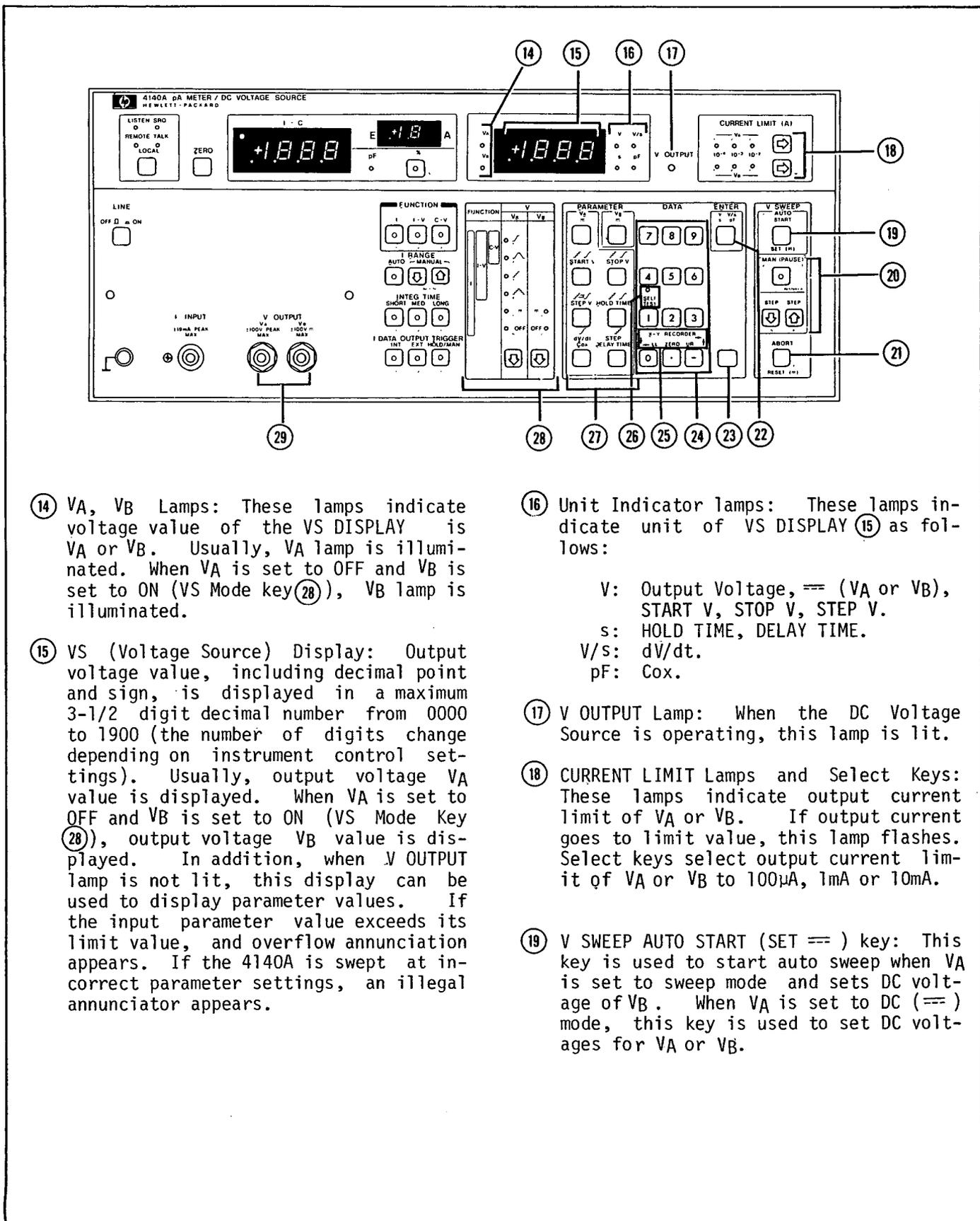
⑭ VA, VB Lamps: These lamps indicate voltage value of the VS DISPLAY is VA or VB. Usually, VA lamp is illuminated. When VA is set to OFF and VB is set to ON (VS Mode key ⑳), VB lamp is illuminated.
