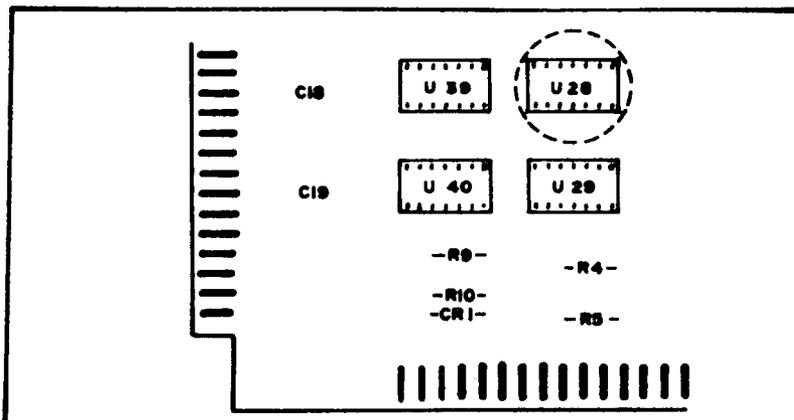
Figure B. Part of A4 Board Component Locations.
