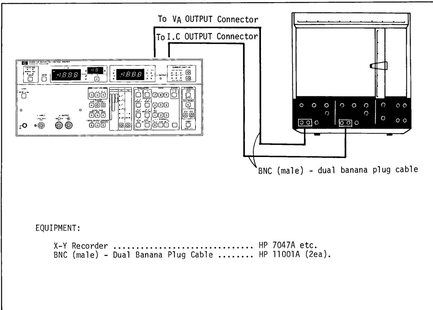
Figure 3-24. Option 001 Analog Output Operating Instructions (sheet 1 of 2).
