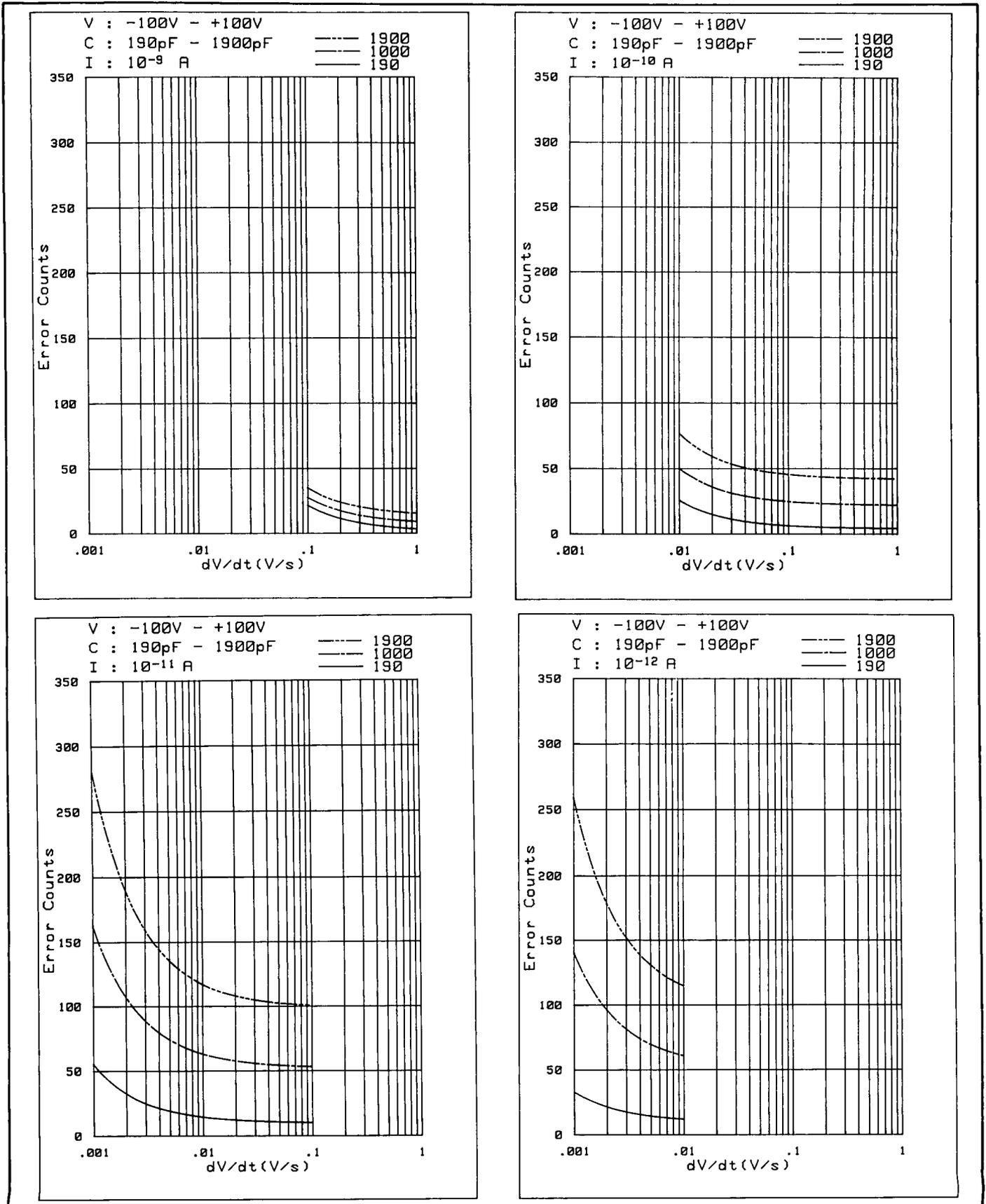
Figure 3-22. C-V Measurement Accuracy (Sheet 4 of 4).
