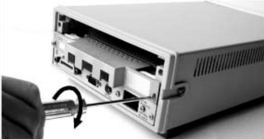
1. Push firmly until the terminal block “snaps” into place.
