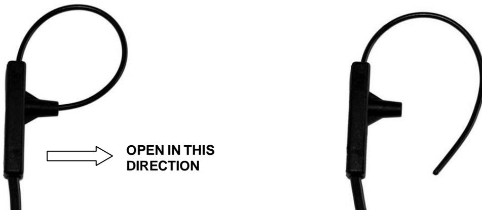
When clipping or unclipping the coil, hold the ferrule as shown
