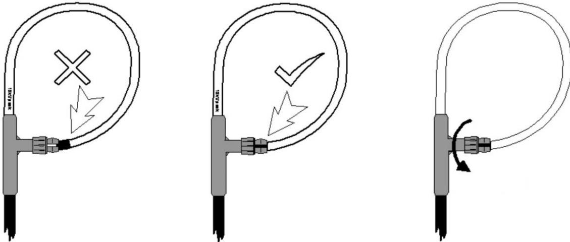
Once the free end of the coil is fully engaged in the ferrule, turn the ferrule lock nut to lock the coil end in position.
